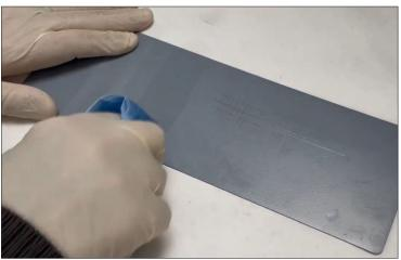
Have you ever been applying a coating out in the field and wanted to know if enough time had passed to apply the topcoat? Our newest demo video shows how to do a quick solvent rub test to make sure your coating has cured.
