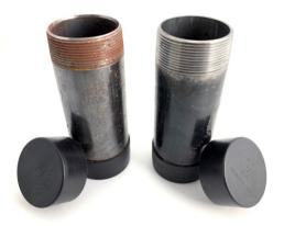
together. During humidity testing, pipe threads capped with a CorroLogic<sup>®</sup> CorrPlug<sup>®</sup> showed a significant advantage in corrosion protection compared to pipes capped with regular plastic containing no corrosion inhibitors.
