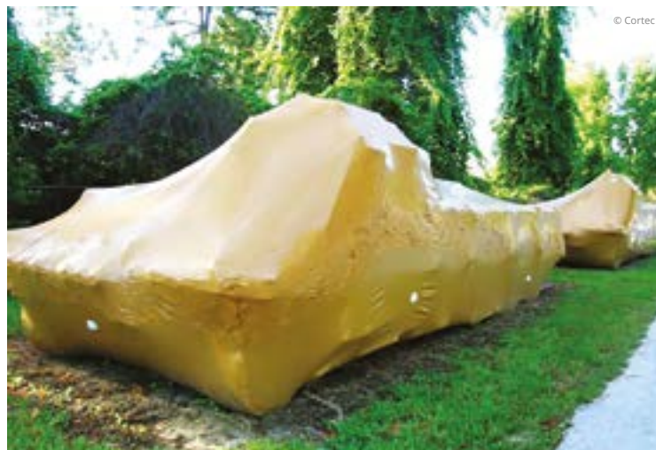
Figures 3 and 4 - Examples of military vehicles packed with MilCorr FR VpCI Shrink Film.
