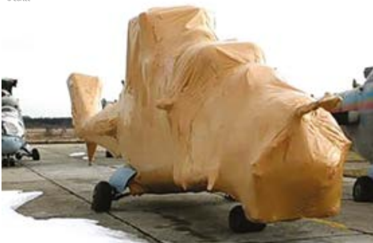
Figures 3 and 4 - Examples of military vehicles packed with MilCorr FR VpCI Shrink Film.
