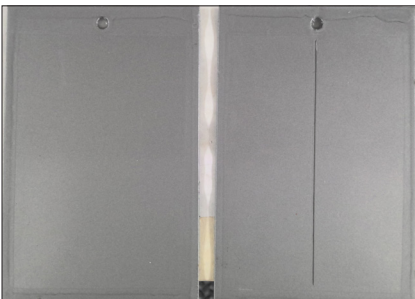
Oxidized panels after being cleaned, coated with VpCI®-373/VpCI®-395/EcoShield® VpCI®-386 Aluminum, and subjected to 1,000 hours in salt fog.
