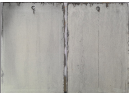
Oxidized panels after being cleaned, coated with VpCI®-373/VpCI®-395/VpCI®-384 Clear, and subjected to 1,000 hours in salt fog chamber.
