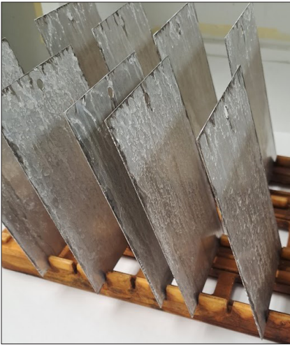
Oxidized aluminum panels after 500 hours in salt fog chamber.
