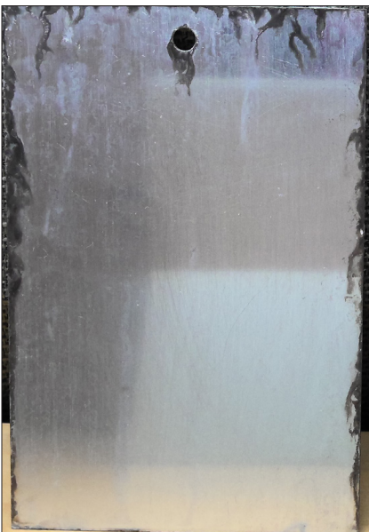
Oxidized aluminum panel after oxide removal with VpCI®-426 and cleaning with VpCI®-415.
