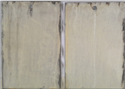
Oxidized panels after being cleaned, coated with VpCI®-373/VpCI®-395/EcoShield® VpCI®-386 Clear, and subjected to 1,000 hours in salt fog.
