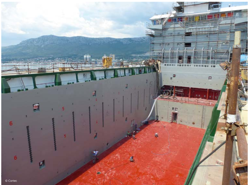
M-645 is ideal for ballast tanks that are frequently emptied and refilled as well as hydrostatic testing applications. Typical applications of M-645 float coat include hydrostatic testing of pipelines, vessels, and ASTs, and seawater ballasting of ships, buoys, and oil rigs.
