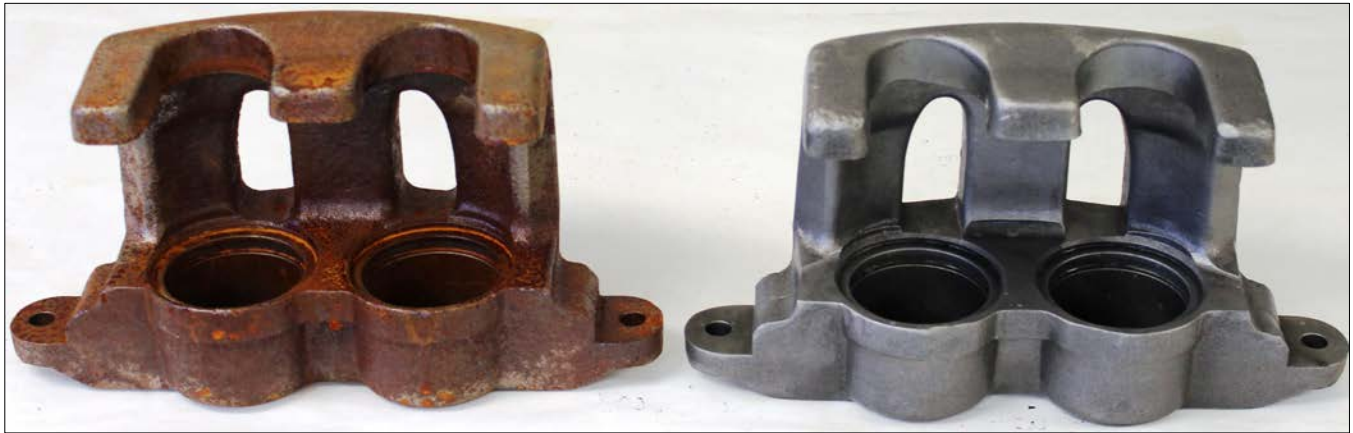
Non-toxic rust removers such as VpCI®-422 can effectively clean the rust off parts to restore them to usable condition on the same day.
