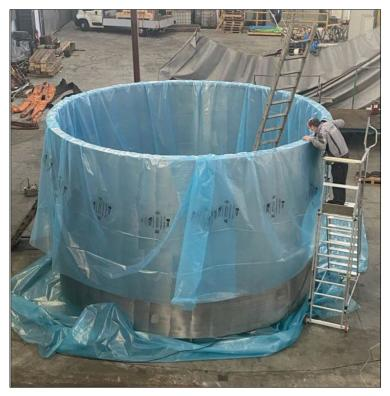
turbine shafts, rings, and hubs. In addition to a protective coating on some of the most sensitive parts, the components needed this heavy-duty VpCI<sup>®</sup> Film for two to five years of storage, possibly outdoors.
