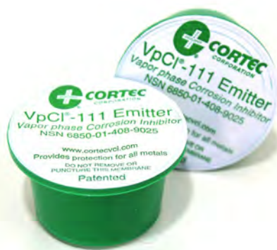
Figure 1: VCI Emitters Contain Corrosion Inhibitors That Vaporize and Condense in a Protective Layer on Metal Surfaces When Placed Inside Enclosures Such as Electrical Cabinets (Source: Cortec Corporation).
