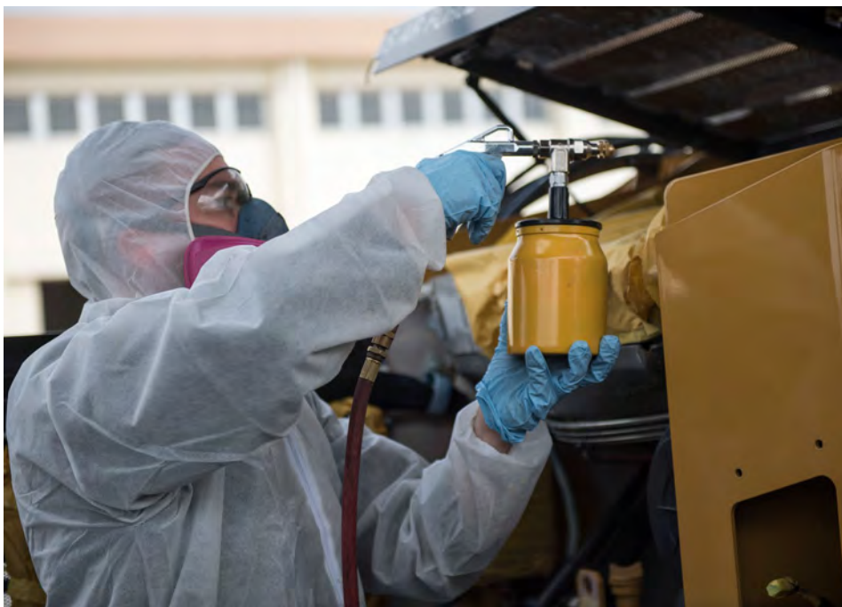
Figure 2: Personal Protective Equipment and Good Surface Prep Are Two Important Aspects of a Safe and Effective Coatings Application (Source: Senior Airman Omari Bernard, 18 th Wing Public Affairs).
