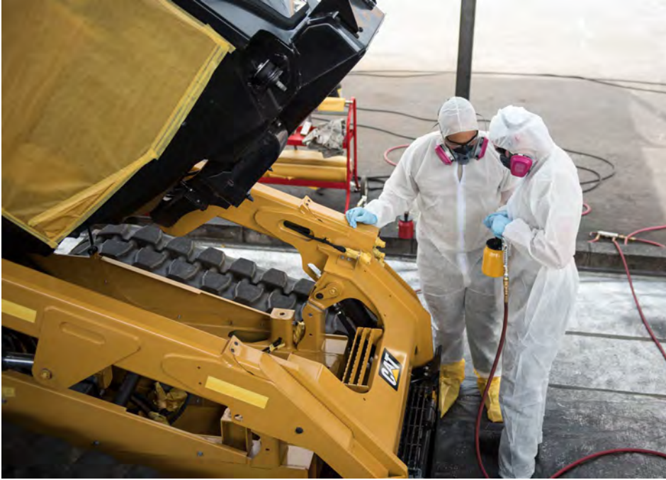
Figure 4: Two Members of the 18 th Logistics Readiness Squadron Prepare to Apply Corrosion Inhibitor Coatings After Having Masked Off Critical Areas (Source: Senior Airman Omari Bernard, 18 th Wing Public Affairs).
