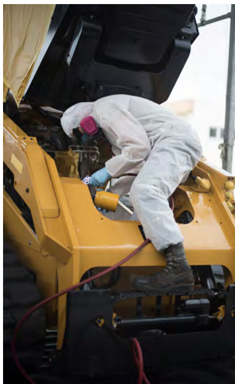
Figure 3: Spraying Coatings Inside Engine Compartment to Provide Extra Protection Against the Corrosive Environment (Source: Senior Airman Omari Bernard, 18 th Wing Public Affairs).
