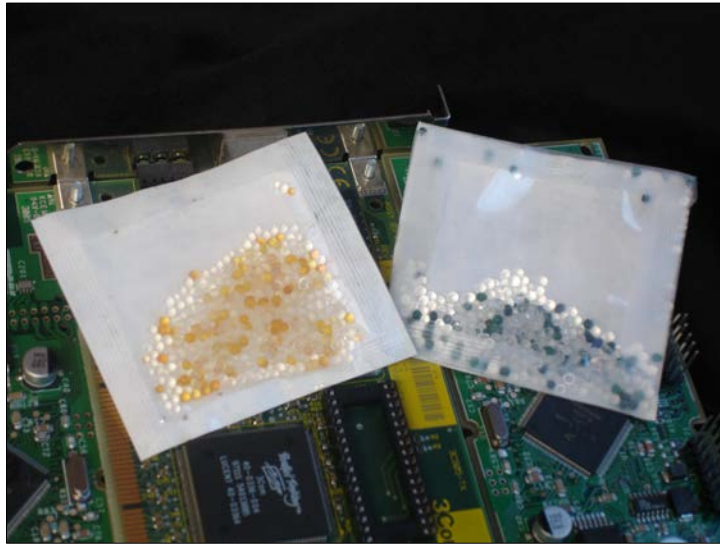
The windowed version shows the indicator spheres that change color when the desiccant is fully spent.
