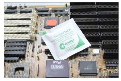
Unlike conventional desiccants, the dual function of Desicorr® VpCI® Pouches/NW reduces moisture in the air (desiccant action) and provides multi-metal corrosion protection (VpCI® action) within a package. In essence, the desiccant action allows the VpCI® to have free access to the surface of the metal, without competition from moisture on the metal surface. VpCI® molecules in the pouch vaporize, emit through the
