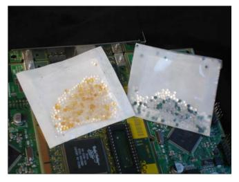
This synergistic action between desiccant and VpCI® provides unparalleled corrosion protection. Even when the desiccant is fully spent, the VpCI® continues to provide corrosion protection and replenish the protective layer on metal surfaces after the package is opened and resealed. This protective layer automatically evaporates when the end user removes the protected product from the package. Unlike many traditional rust preventatives, no degreasing or
