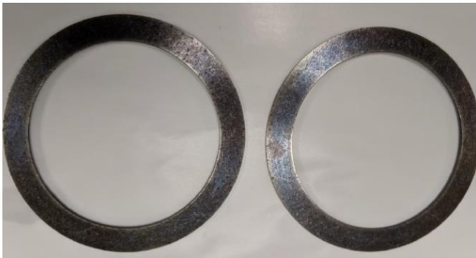
Figure 4: Close up of parts protected by yellow VCI film and silica desiccant. Small dark spots of corrosion starting can be seen along the top surfaces.
