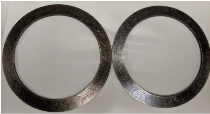
Figure 3: Close up of parts protected by VpCl-126 and DesiCorr. No signs of corrosion.
