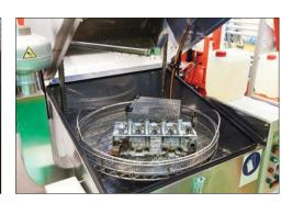
Maintenance of dip tank health is an important task for anyone using Cortec® products in a dip bath or recirculating application. As the rust preventative, cleaner, hydrotesting additive, or other product is used over time, it will gradually decrease in strength and volume. Products may also become contaminated through improper storage or the buildup of dirt, grease, or machining oils from the metals dipped in the tank. In either case, the product becomes less effective.
