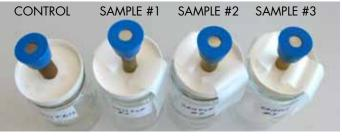
VIA Test: Conforms to MIL-PRF-22019D
