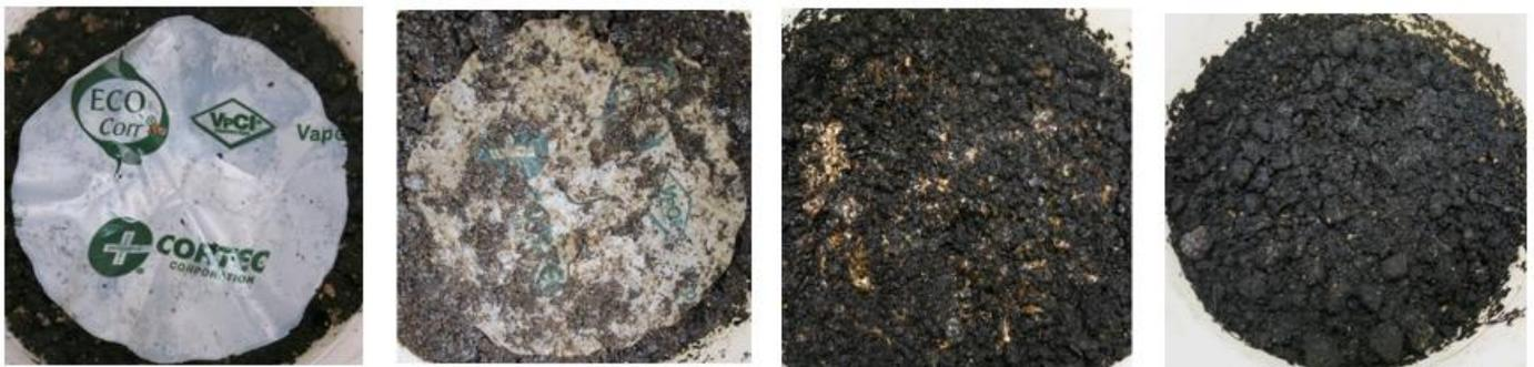
Biodegradation process of EcoCorr® lasts up to 10 weeks.
