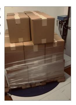
Eco Wrap<sup>®</sup> is extremely elastic and works on most existing automated machines, simply by adjusting (typically increasing) the tension.
