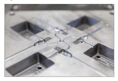
After cleaning, additional corrosion protection may be needed depending on when and how the component will be used, stored, or shipped. For example, newly made dies or plastic-injection molds can be protected by spraying the mold internals with EcoAir® Tool & Die Rust Preventative. EcoAir® Tool & Die is partially based on vegetable oil and leaves a water-displacing film on metals. EcoAir® spray-can
