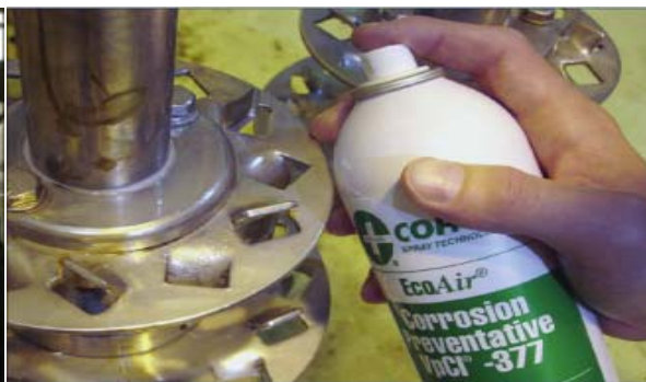
EcoAir® Corrosion Preventative, VpCI®-377 provides multi-metal corrosion protection indoors forming a clean, dry, hydrophobic film
