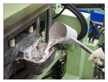
Cortec's new EcoAir® Mold Release provides dual protection for these needs by combining lubrication with a biobased corrosion inhibitor for injection molds and other metal surfaces. When sprayed on the mold, EcoAir® Mold Release leaves a clear thin non-staining silicone coating that makes it easier to release rubber, plastic, or metal castings from their molds. The biobased corrosion inhibitor
