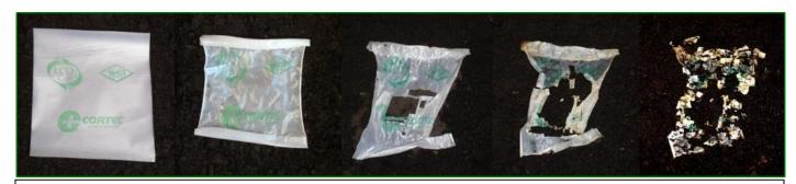
Eco-Corr Film disintegrates into carbon dioxide and water within months in a commercial composting environment.
