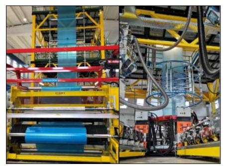
The plant has two production halls. Together with new offices, the brand new 2000 square meter facility also includes state-of-theart extrusion line E5. EcoCortec<sup>®</sup> has sideweld and bottomweld converting machines for making a wide range of bags. Film rewinder and recycling equipment allows elimination of waste from the production process. The plant's
