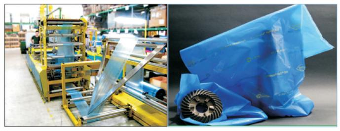
New converting line and termal transfer printing capabilities enable EcoCortec® to produce short runs of high quality patented EcoShield VpCl®-226 and Corrshield VpCl®-126 heatsealable and ziplock bags. These films protect metal parts from all types of corrosion including rust, tarnish, stains, white rust and oxidation for up to 5 years.
