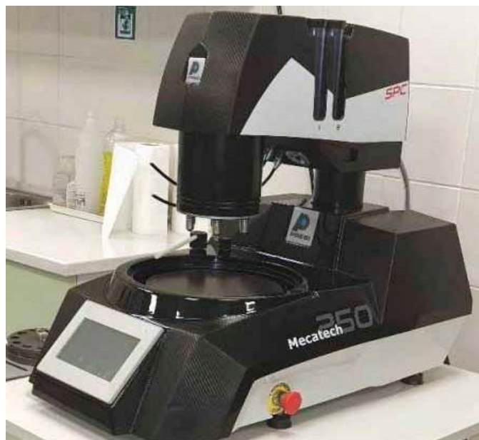
Plug polisher for VIA testing according to NACE TM-0208 or Cortec® method.
