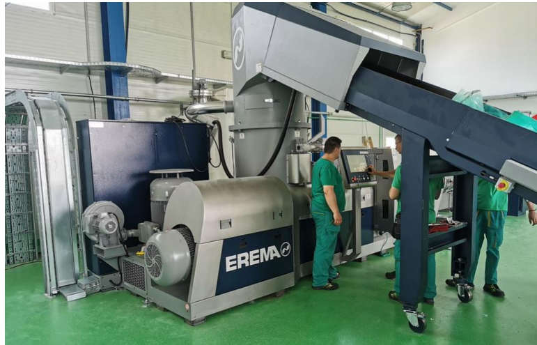
New Erema reggranulation machine reprocesses plastic scrap and waste onsite.
