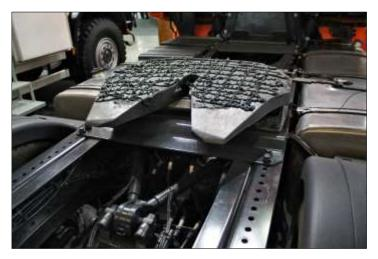
sliding or rolling metal-to-metal contact areas such as trailer hitches or other mechanical joints.
