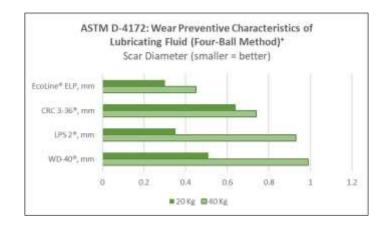
When tested according to ASTM D-4172 Wear Preventive Characteristics of Lubricating Fluid (Four-Ball Method), EcoLine<sup>®</sup> ELP showed a much smaller scar diameter than the three other products.
