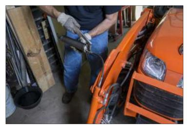
EcoLine<sup>®</sup> Heavy Duty Grease is a premium quality biobased, biodegradable grease for extreme pressure applications. It is formulated with a vegetable-oil base, lithium-complex-based thickener, and extreme pressure additives for superior lubricity and maximum performance under heavy loads. EcoLine<sup>®</sup> Heavy
