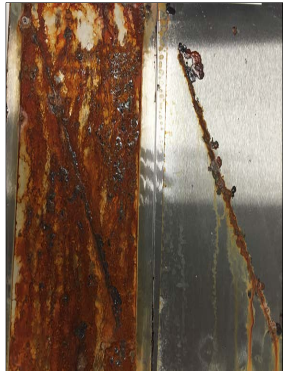
On Left: Traditional Water Based Coating at 1 Mil. At Right: Cortec's EcoShield® 386 Water Based Coating Powered by Nano VpCI®.
