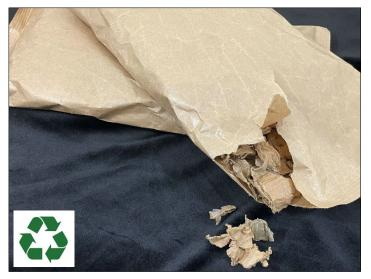
A new idea to recycle the corrugated box waste into something valuable onsite was investigated. Special processing equipment from Europe along with a packaging machine from PAC Machinery's sister company, Audion, allowed the facility to chop up used cardboard boxes and automatically pack them inside paper bags made on an adjacent AVM vertical form, fill, and seal machine. These "dunnage bags" could then be placed inside shipping boxes for cushioning and void space fill.
