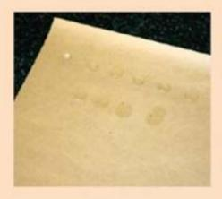
through in the same time frame, at the higher rate of 0.47-0.71 grams per hour. The waxed paper was much less resistant to water vapor, allowing it to transfer at a rate of 6.5-6.9 grams per hour on the same size of paper. Though it is not intended for applications involving constant water contact, the shiny side of EcoShield also has the ability to repel liquid water. Its TAPPI T-441 Cobb water absorption rate is less than 0.3 grams of water per square meter in 2 minutes.
