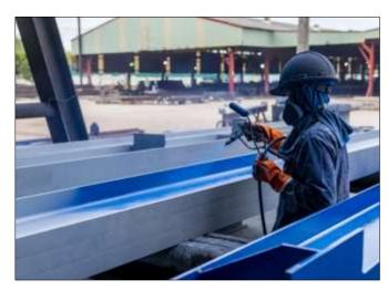
steel, EcoShield® 386 can be tinted to match the facility color scheme or to stand out in bright safety colors. As an added advantage, EcoShield® 386 is weldable, allowing OEMs to apply corrosion protection right off the production line to tubing or other metals that need to maintain a rust-free surface for later welding.
