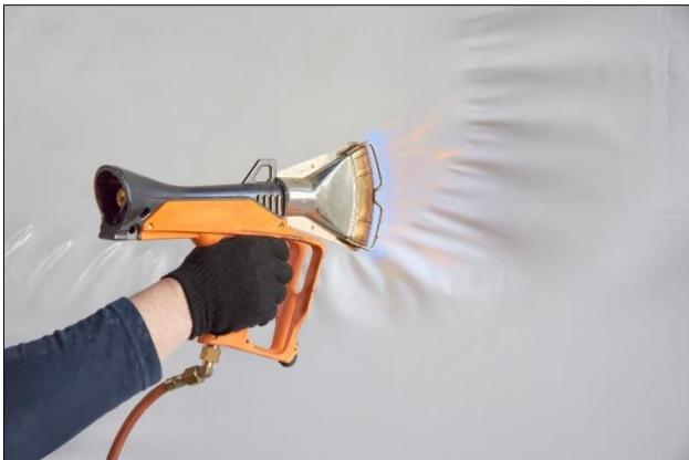
EcoShrink™ has many practical characteristics in addition to being environmentally safe. Film is specially designed for standard heat-shrinking applications. Cortec’s customers can shrink wrap their small or large components as normal to conform to the shape of the object. EcoShrink™ is an excellent way to keep dust, dirt, and moisture off warehouse stock while keeping components bundled into a streamlined package.
