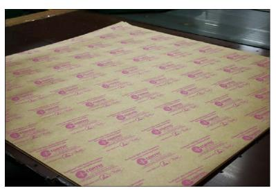
typical imidazolines, phosphated esters, and nonionic based antistat coatings. The antistat protection from EcoSonic® ESD Paper is thermally stable at high temperatures (in excess of 392°F (200°C) and pH stable between 2 and 11 at temperatures in excess of 100°F (38°C) for several days. EcoSonic® ESD Paper conforms to performance specifications for MIL-PRF-81705D (Static Decay Rate and Surface Resistivity).
