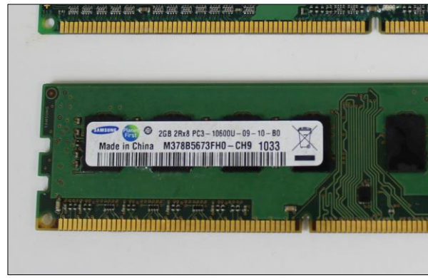
ElectriCorr VpCI-239 after 90 hours salt spray
