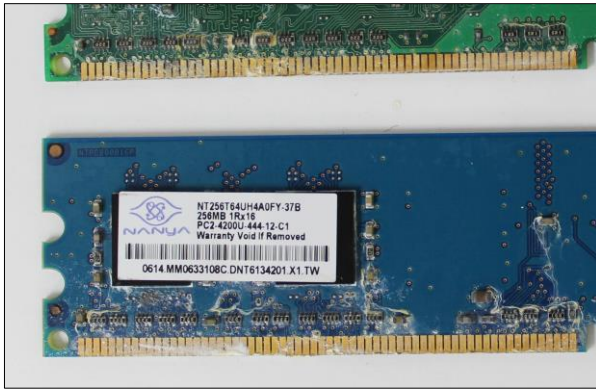
Control - Close up after 90 hours salt spray
