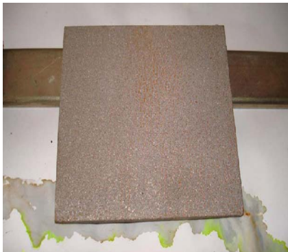
The sample in water treated with 0.4% VpCI 645. After 24 hours of immersion in water and drying the air - a satisfactory result is achieved with a half of the recommended concentration.
