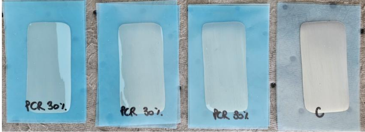
Figure 1: Razor Blade Test- Carbon Steel for sample VCI PCR 30% at the beginning (left) and end (right) of the test.
