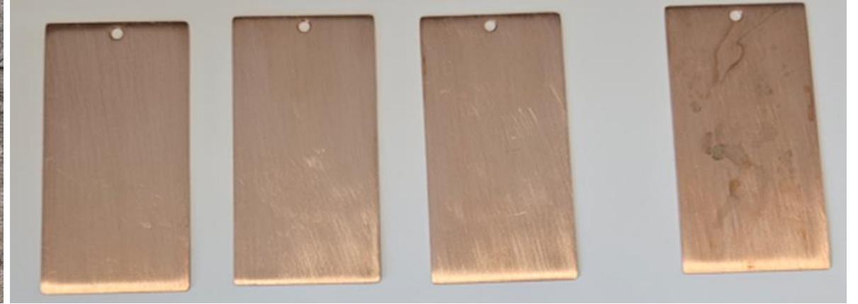
Figure 1: Razor Blade Test- Cooper for sample VCI PCR 30% at the beginning (left) and end (right) of the test.
