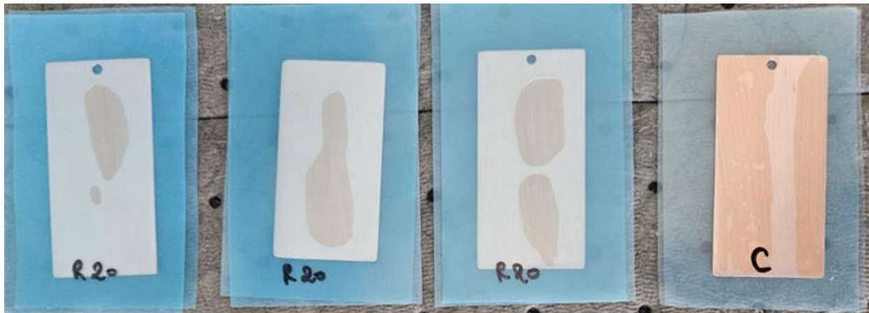
Figure 2: Razor Blade Test- Cooper for sample VCI PIR 20% at the beginning (left) and end (right) of the test.
