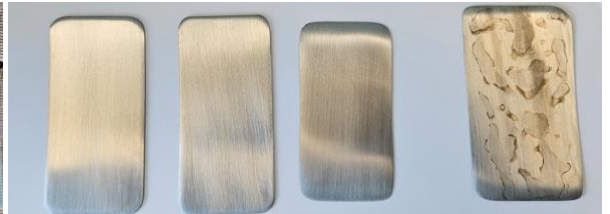
Figure 2: Razor Blade Test- Carbon Steel for sample VCI PIR 20% at the beginning (left) and end (right) of the test.
