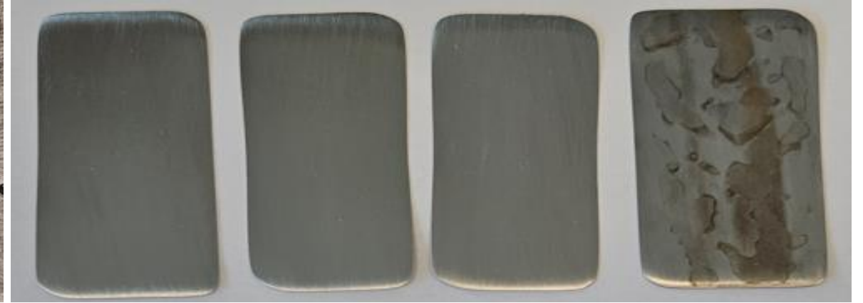
Figure 1: Razor Blade Test- Carbon Steel for sample VCI PCR 30% at the beginning (left) and end (right) of the test.
