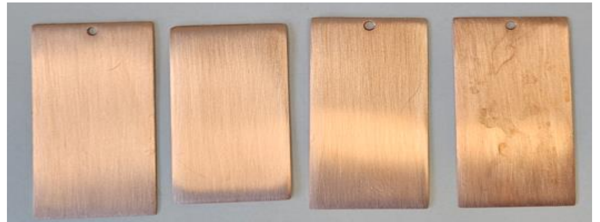
Figure 2: Razor Blade Test- Cooper for sample VCI PIR 20% at the beginning (left) and end (right) of the test.
