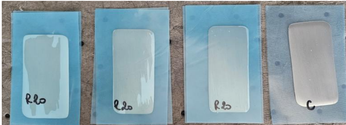
Figure 2: Razor Blade Test- Carbon Steel for sample VCI PIR 20% at the beginning (left) and end (right) of the test.
