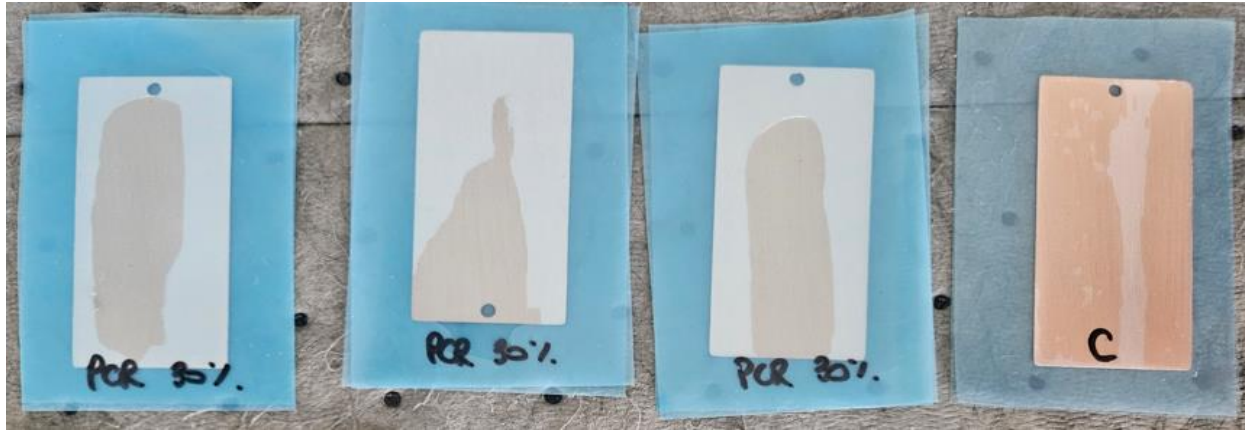
Figure 1: Razor Blade Test- Cooper for sample VCI PCR 30% at the beginning (left) and end (right) of the test.
