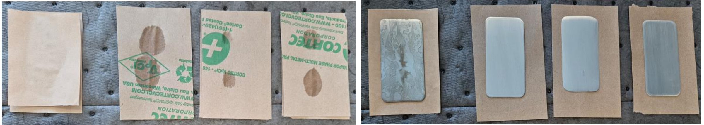
Figure 2: Razor Blade Test- Carbon Steel for sample VCI paper at the beginning (left) and end (right) of the test.
