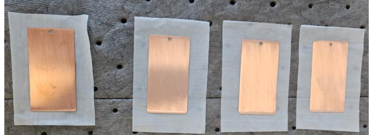
Figure 3: Razor Blade Test- Cooper for sample biodegradable VCI ESD film at the beginning (left) and end (right) of the test.
