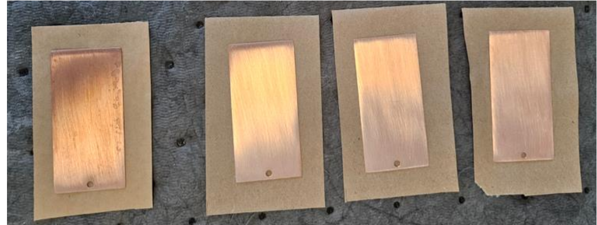
Figure 4: Razor Blade Test- Cooper for sample VCI paper at the beginning (left) and end (right) of the test.
