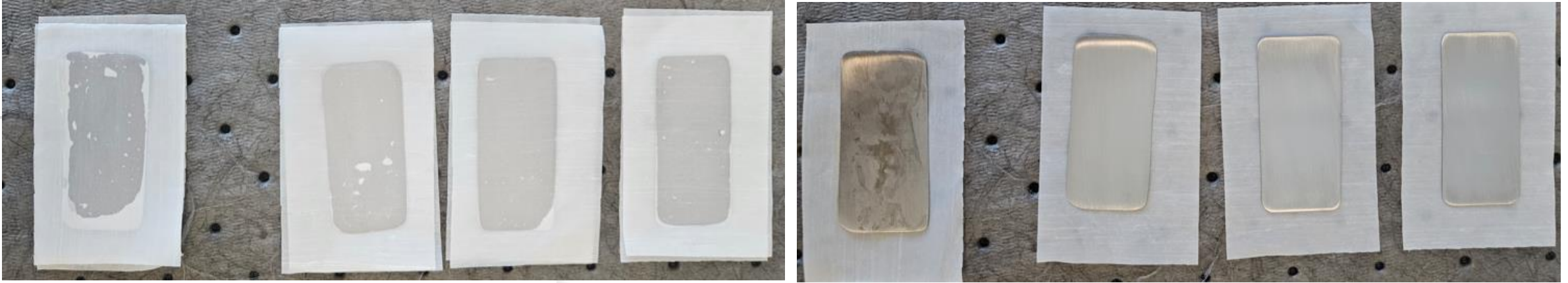
Figure 1: Razor Blade Test- Carbon Steel for sample biodegradable VCI ESD film at the beginning (left) and end (right) of the test.
