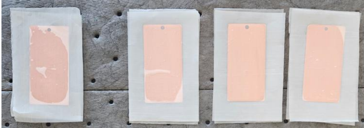
Figure 3: Razor Blade Test- Cooper for sample biodegradable VCI ESD film at the beginning (left) and end (right) of the test.
