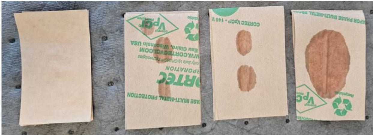
Figure 4: Razor Blade Test- Cooper for sample VCI paper at the beginning (left) and end (right) of the test.
