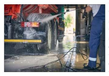
While it is ideal to target corrosion at its root source by adding a corrosion inhibitor directly to the deicing salt, the most effective protection is often regular washing after a vehicle outing. Leaving a vehicle to sit unwashed after driving around on winter roads, caked with chloride-rich road spray that has splashed up on the sides and bottom of the truck or car, is one of the quickest routes to rusting out a vehicle. Simple washing goes a long way toward removing chlorides
