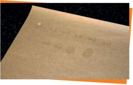
50% relative humidity. The Eco-Shield<sup>®</sup> Super Barrier Paper and Linerboard showed a water vapor transfer rate of 0.32-0.37 grams per hour on a square meter of paper. A polycoated paper in the same test allowed slightly more water vapor to pass through in the same time frame, at the higher rate of 0.47-0.71 grams per hour.
