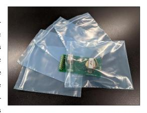
into one bag, Cortec® reduces the need to add desiccant, streamlining the electronics packaging process. Avionics that are not static sensitive can likewise benefit from VpCI®-126 bags, which provide corrosion protection minus the ESD protection and desiccant. With these solutions, avionics manufacturers and distributors have some great options to cope with uncontrolled shipping and storage environments on many types of avionics:
