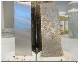
After one day. No corrosion was found on the panel from the jar with  $VpCI^{\textcircled{R}}$ -609 and ~ 95% of the surface of the panel was corroded in the 'Control' jar.
