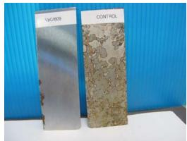
Panels after 2 weeks in sand. According to the test results  $\rm VpC1^{\textcircled{\$}}$ -609 provides excellent corrosion protection in the sand saturated with the submitted water sample
