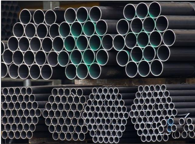
This was the case with a manufacturer who needed an anticorrosion coating to protect the outer diameter (OD) of steel pipes from corrosion until commissioning by the end user. Manufacturer requirements were very rigorous, demanding protection at 1 mil DFT (dry film thickness) and compliance to stringent VOC standards. In addition, the coating needed good hot hardness so the pipes would not stick together after force-drying. This also
