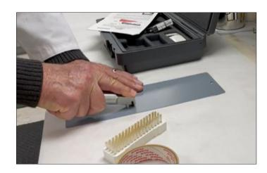
We are pleased to release a new demo video on how to test coating adhesion! This test can be very important for coating applicators who want to make sure their first coat of paint has cured enough to apply the second coat—or for applicators who simply want to paint over an old coating. Good coating adhesion is critical to the success of an anticorrosion coating system because if the coating does not stick to the surface, protection is lost. If adhesion is good, the coating can do its job!
