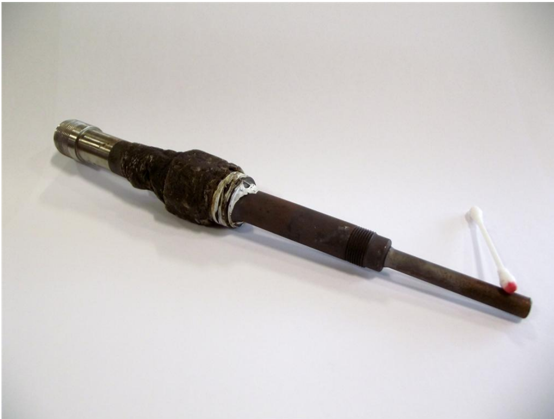
Figure 4: Positive inhibitor test on the sensor end of a corrosion probe.
