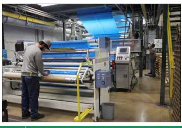
After it is printed with the Cortec® logo and QR code, the film runs through a new high-tech winder that improves productivity by reducing scrap and labor. It is also an important improvement in workplace safety. Previously, CAF had to have two operators on the machine as an extra safeguard against accidents. With the new technology, CAF is able to move one of those operators to a different task, cutting labor costs in half.
