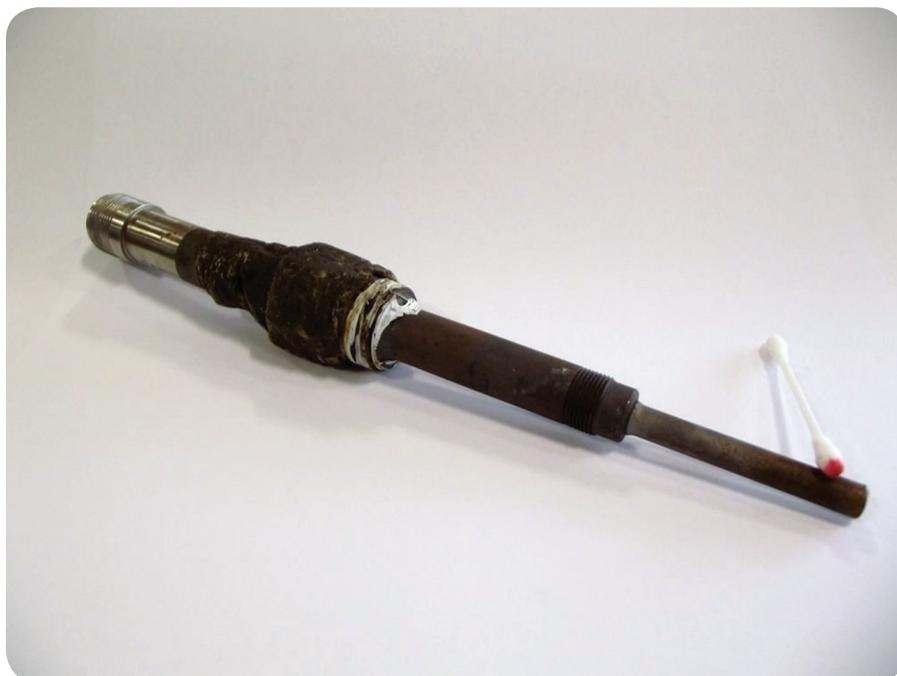
**FIGURE 5** The sensor end of a corrosion probe tested positive for the inhibitor.
