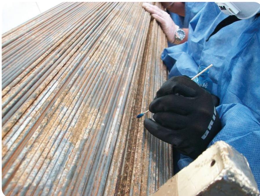
**FIGURE 4** A swab test for the presence of inhibitor was done during cable inspection.
