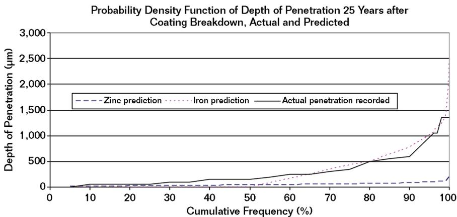
**FIGURE 2** Comparison between actual and predicted depth of corrosion penetration.
