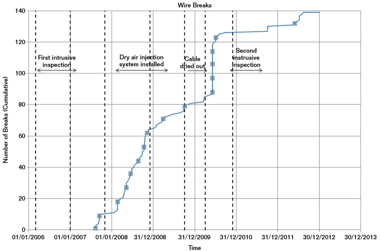
FIGURE 6 Results from acoustic monitoring of the cables.
