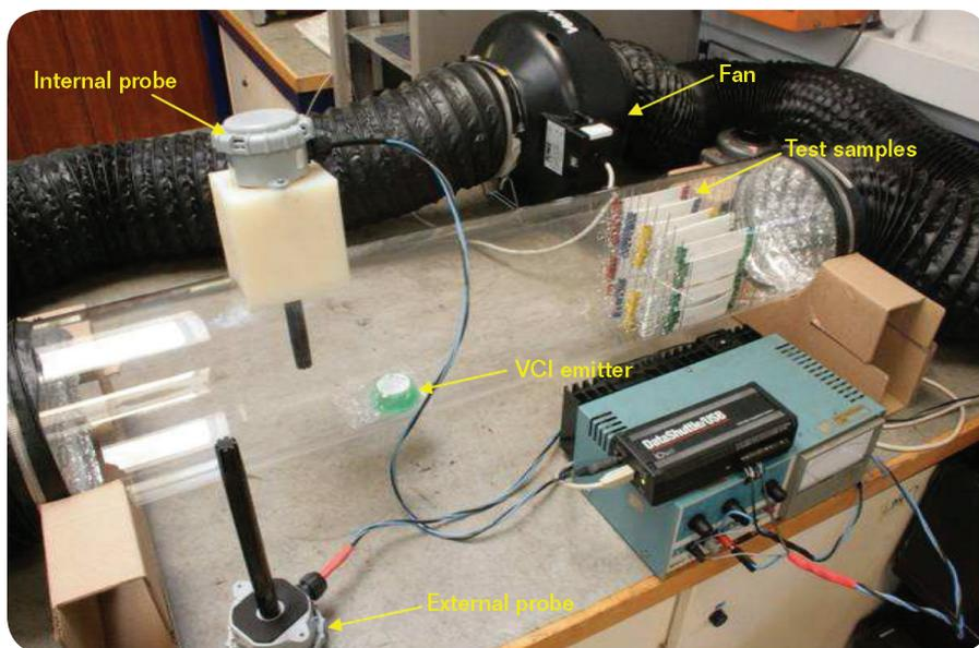
**FIGURE 3** Laboratory tests confirm compatibility of the inhibitor with the dehumidification system components.
