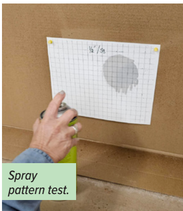
Measuring spray diameter.
