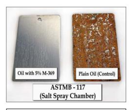
M-369 combines the film-forming properties with Cortec's patented Vapor phase Corrosion Inhibitor (VpCI<sup>™</sup>), which provides protection in places unreachable by film-forming corrosion inhibitors.
