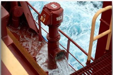
M-645 is ideal for ballast tanks that are frequently emptied and refilled as well as hydrostatic testing applications.
