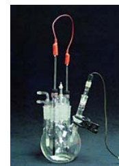
Electrochemical instrumentation used to establish data points that determine corrosion rates.
