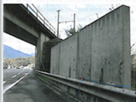
FIGURE 1 Photograph of L-shaped concrete specimens exposed to chloride-containing splash water on a highway in the Swiss Alps.
